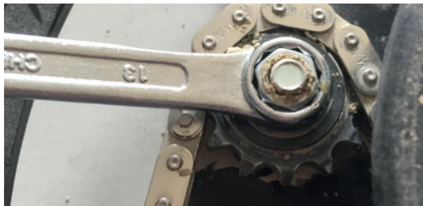
6. Check chain tension, if tension is too weak, repeat procedure.
