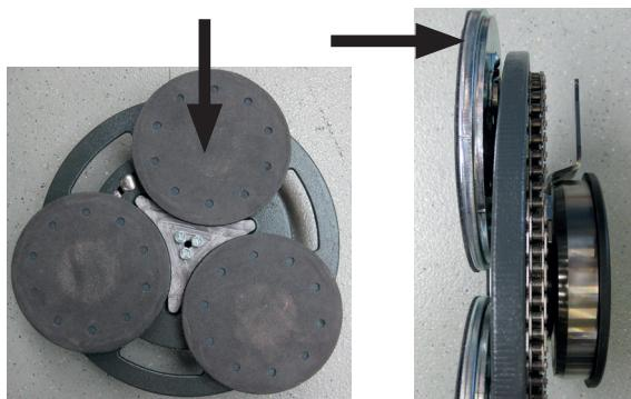
Clean complete **Triple Disc** with compressed air or clean with a damp cloth.
