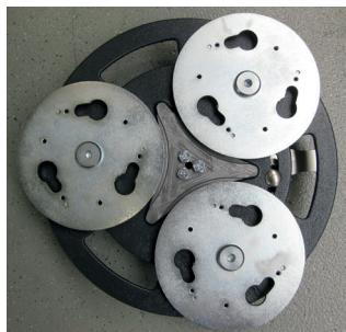
Check **clutch** for damage or heavy contamination.
