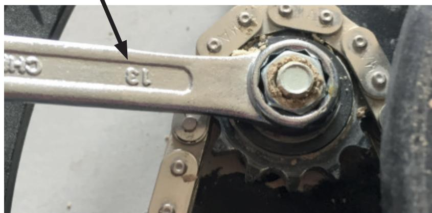
5. Pull the chain tensioning wheel outwards and tighten the nut with the wrench.
