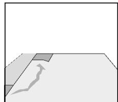
Place the first plank of the new row with the tongue side at an angle against the groove side of the plank in the previous row.
