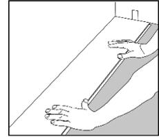
Hold the next plank against the first matching the corners and fold it down until there is a confirming sound of a "click"
