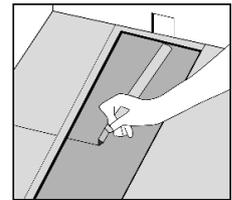
Mark where the plank is to be cut and place it on the work surface and cut to size using any kind of saw.
