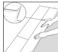
Adjust the distance to the wall to 5mm (0.2") when three rows are complete.
