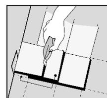
The last and first plank can be cut in the correct width. Place the last plank on top the second to last plank.
