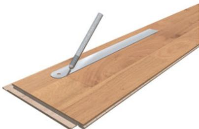
Cut through the acrylic finish layer in the joints around the strip. Use a straight edge.
